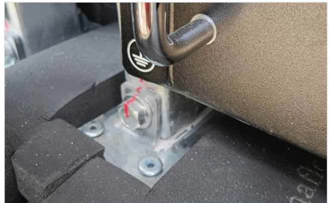
Module mounting bracket, torque witness marks visible
