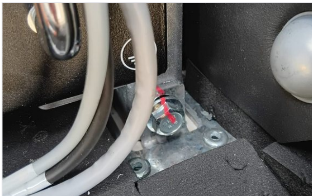
Mounting frame and harness runs, no wiring damage
